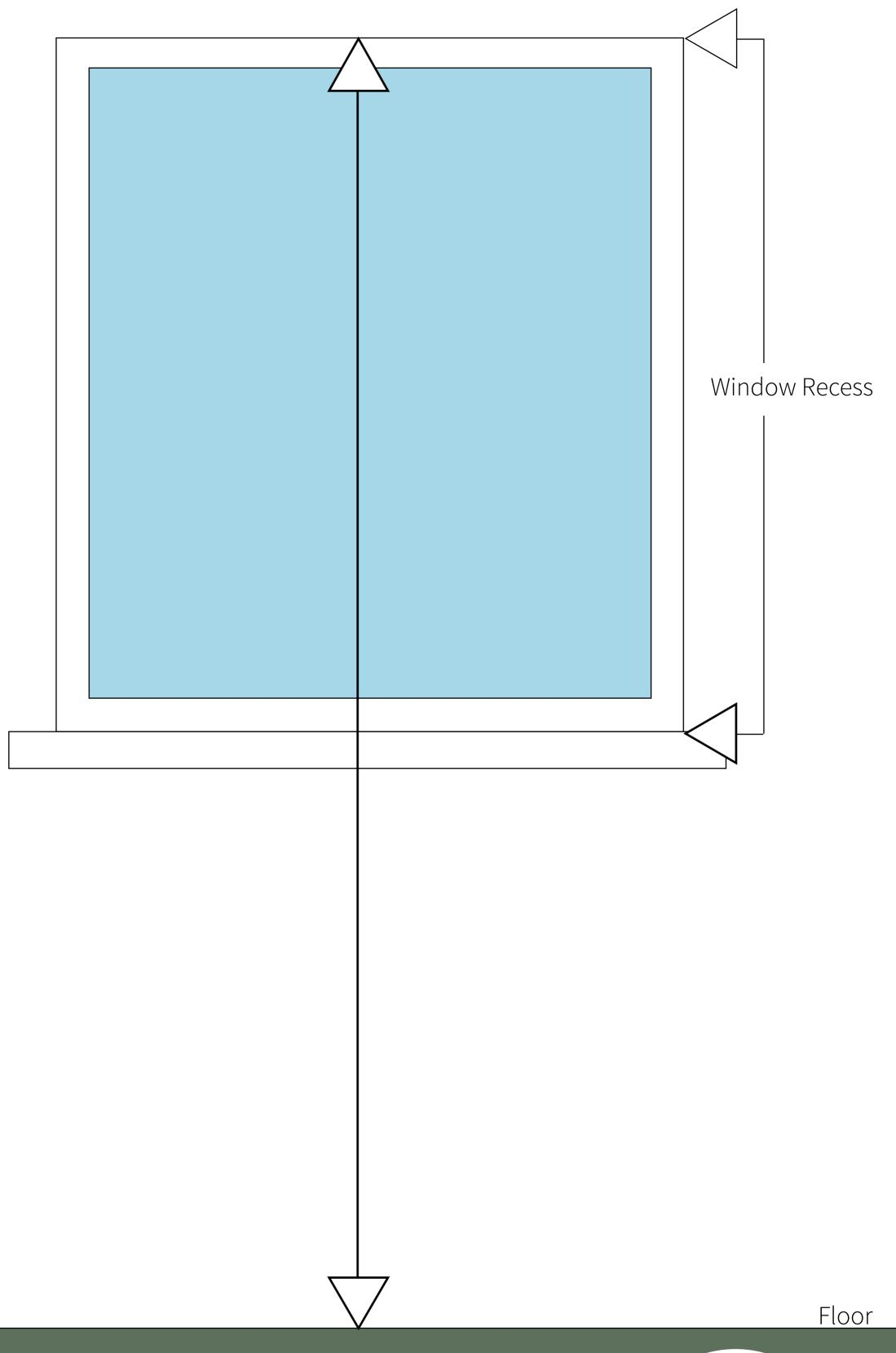
Measure the top of the recess to the floor to ensure the right specifications are applied to your order.
